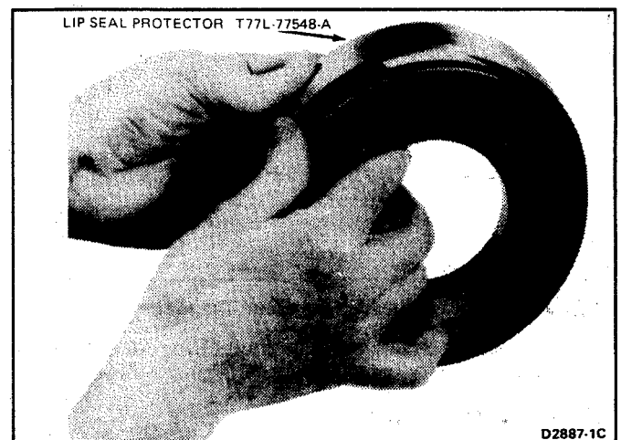
FIG. 52 Installing Forward Clutch Piston and Lip Seal
